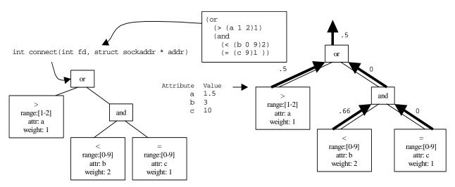
Figure 5: An illustration of constraint parsing and evaluation by the SoNS Interpreter
